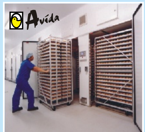
Loading an Avida single-stage setter. Avidas have just one trolley positioned each side of the central paddle fans to ensure that the optimum heating, cooling and ventilation are provided at all times directly and without obstruction.
